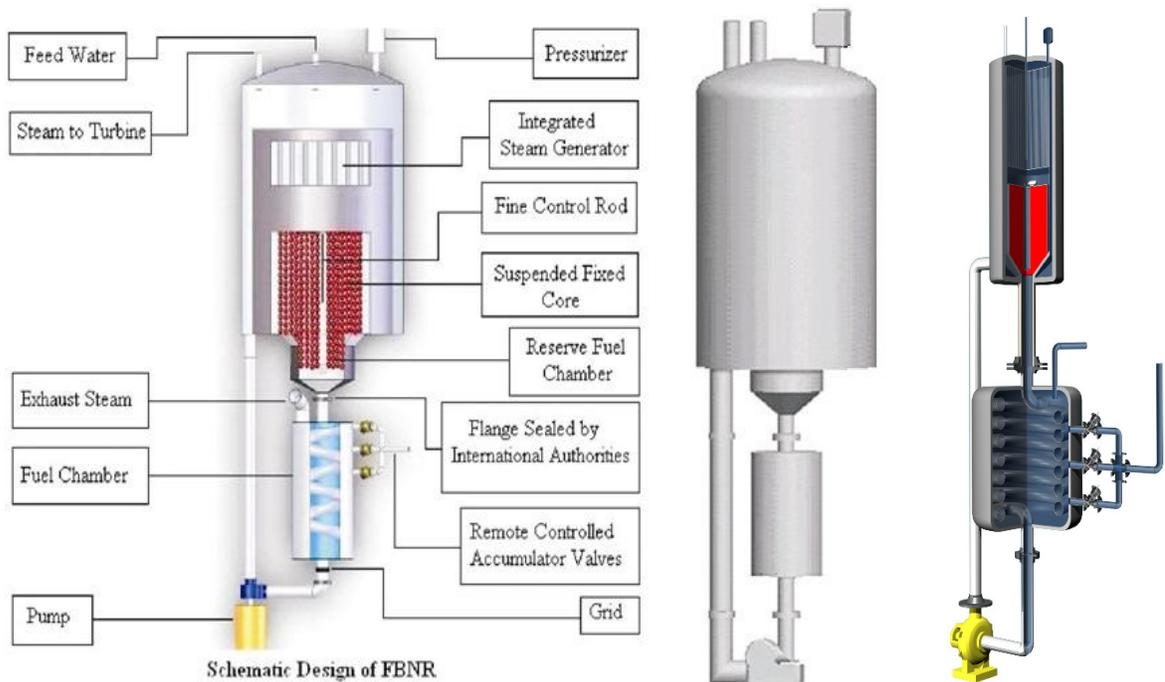
FIG. 2. Schematic Design of the Fixed Bed Nuclear Reactor (FBNR).
