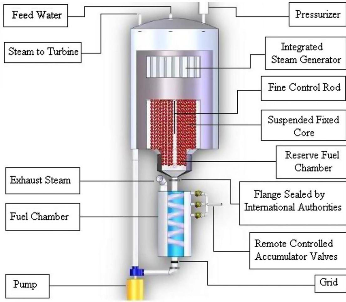
Fig. 1: Schematic design of the main components of FBNR
