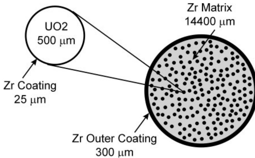
Fig. 2: Cross sectional sketch of the FBNR CERMET fuel
