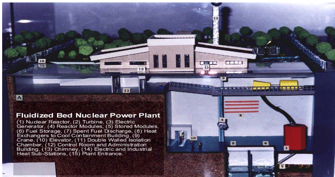
Figure 3. FBNR Underground Containment Building.
