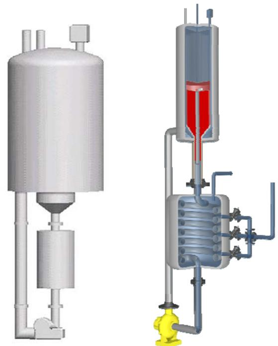
Figure 2. Schematic Design of the Fixed Bed Nuclear Reactor (FBNR).
