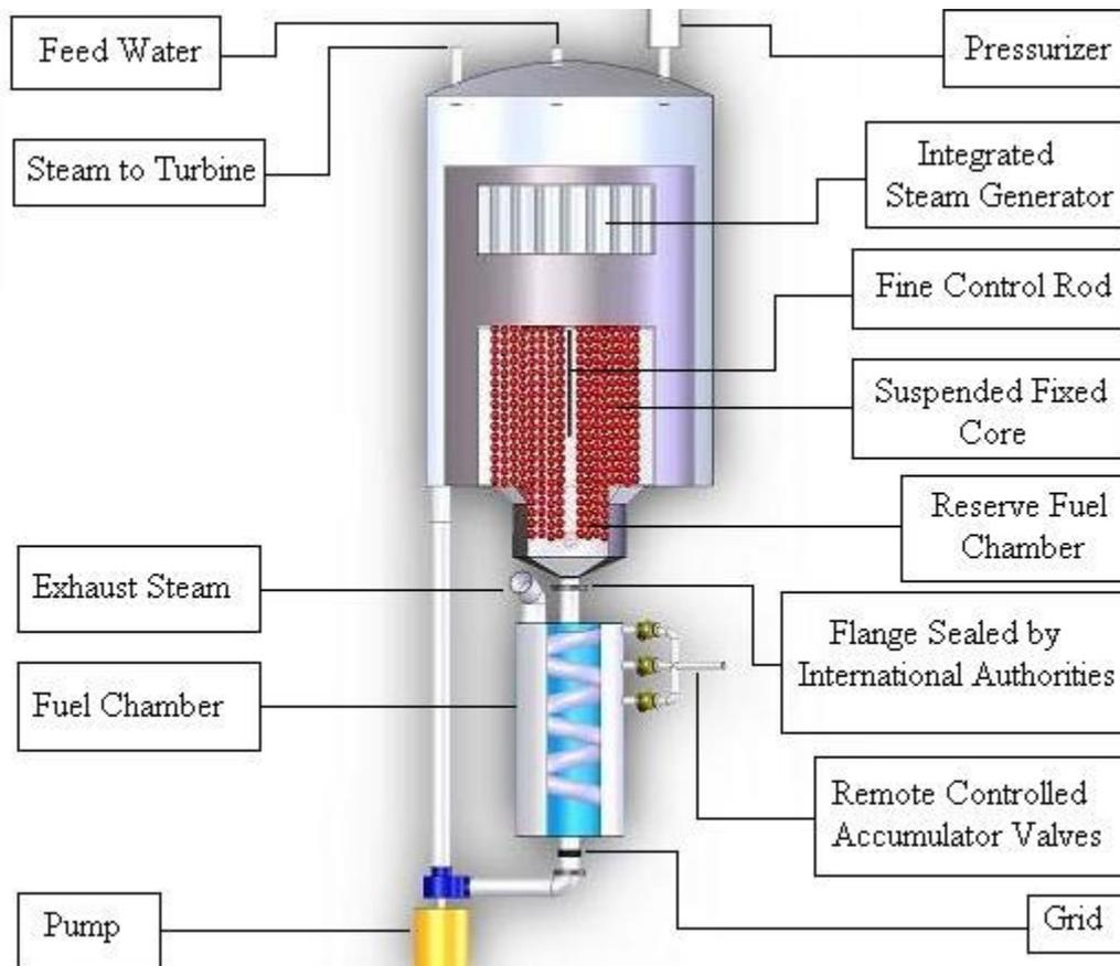
**Figure 1. Schematic design of FBNR**
