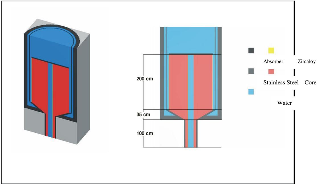
**Figure 3. Keno VI model of homogenous reactor**
