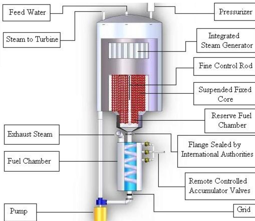
Figure 2-1: Schematic Design of FBNR
