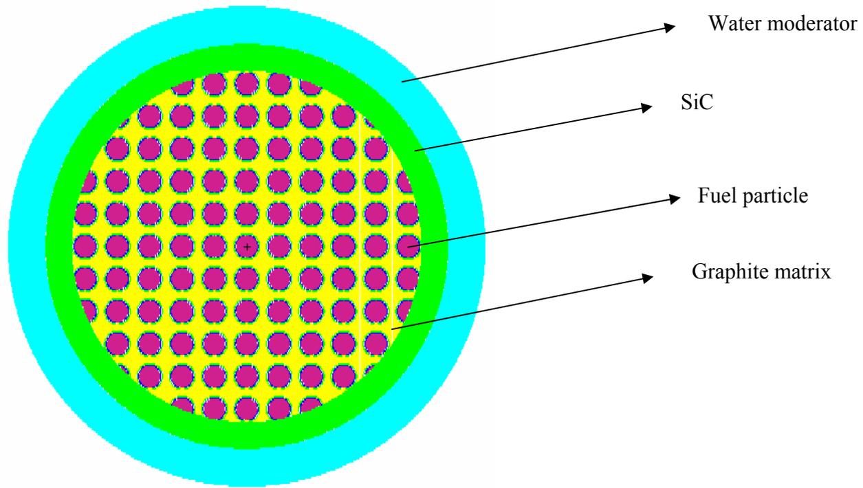
Figure 4: MCNP5 modeling of the FBNR unit cell.
