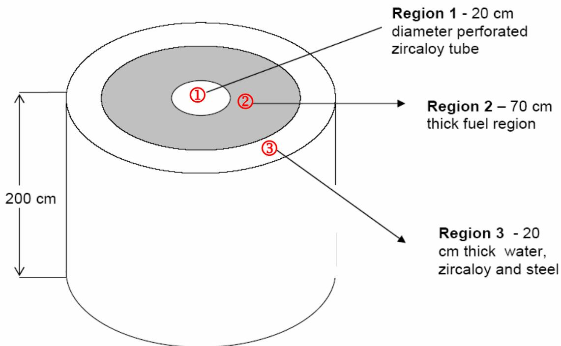
Figure 2: Geometrical modeling of for one dimensional numerical calculations
