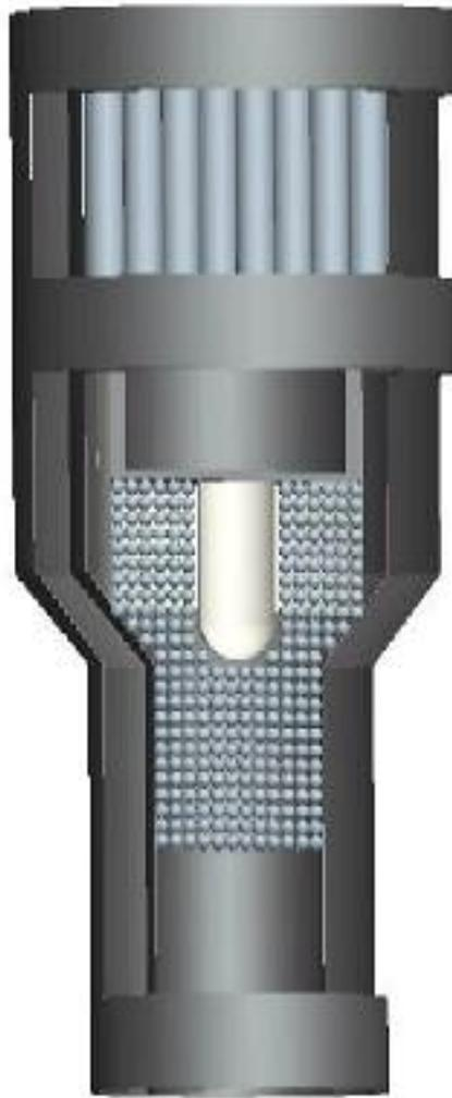
*Operating condition:* The spherical fuel elements are out of the fuel chamber and are in the core. The core level limiter is adjusted allowing sufficient fuel elements enter the core in order to have the reactor in the critical condition. The reserve reactivity is contained in the extra fuel elements that are left in the fuel chamber outside the core.
