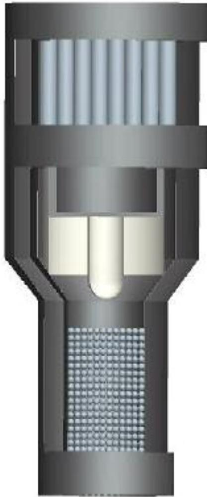
*Shut down condition:* The core is empty and the fuel elements are stored in the passively cooled fuel chamber under a highly subcritical condition. The decay heat is dissipated through natural convection.
