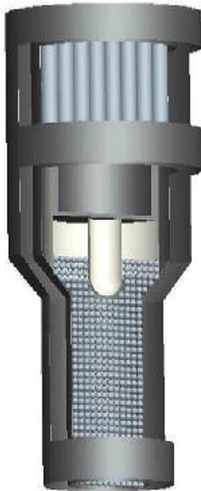
*Shut down or accident conditions:* The pump is turned off automatically; therefore, the fuel elements fall out of the reactor core into the fuel chamber through the force of gravity.
